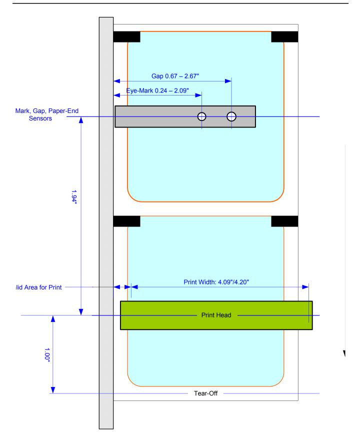
Figure 7-1, Print Setup Dimensions
